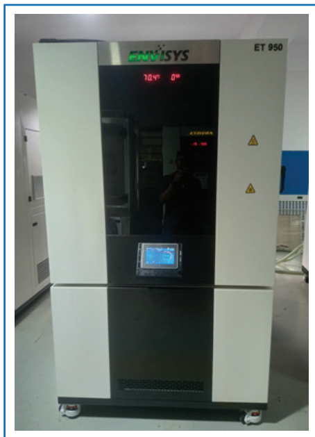
Environmental Test Chamber Temperature range: 40deg c to +180deg c Humidity range: 10%RH -98%RH
