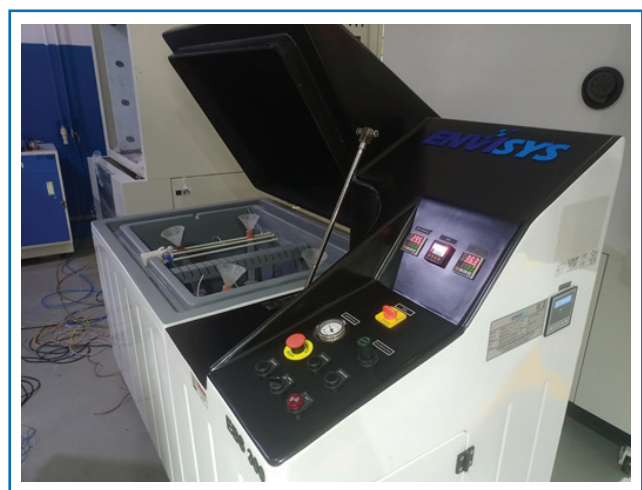
Salt Spray Test Machine Dry cycle: Temp:55deg c Wet Cycle : Temp:55deg c, Humidity:95-100%RH
